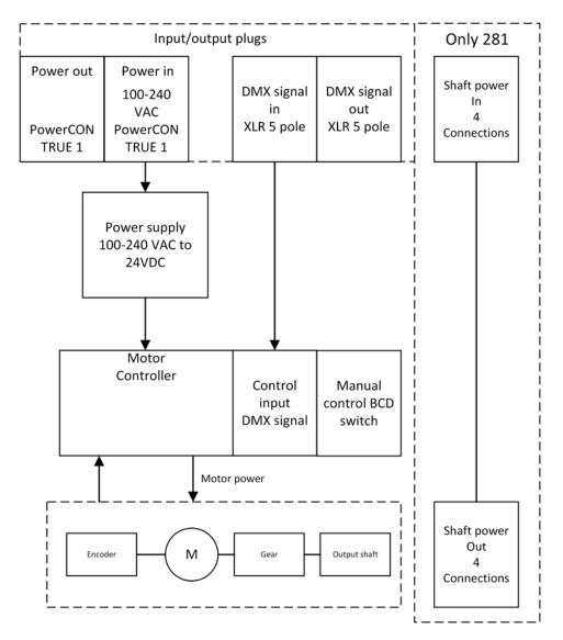
Block diagram of the control system of the Rotator.
