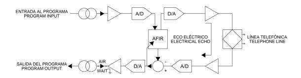
The telephone line is connected to the digital hybrid when you select **T / W** or **AIR** on the keyboard.
