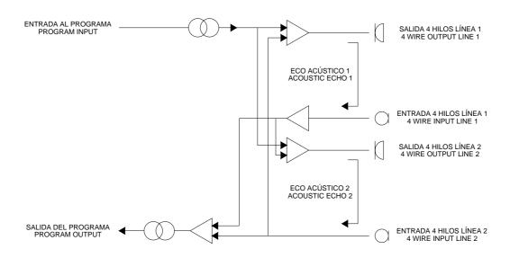
Both intercoms are interconnected through the Mix-Minus bus, and the user of the **AEQ TH-02EX Mk III** can also maintain communication with them. The equipment cancels the acoustic echo generated in each terminal connected to the equipment.
