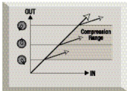
The amount by which the compressor reduces the gain is determined by the 'ratio'. The ratio is conventionally expressed as a numerical value, e.g. '4:1', which represents the amount by which the gain is reduced when the volume of the signal rises above the threshold.
