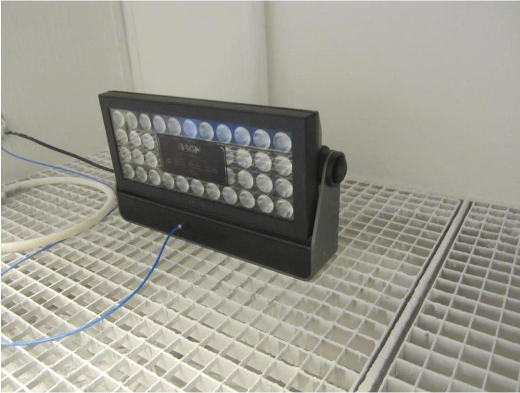
Photo 1. IP6X Test P-5 Wash Light before exposure.
