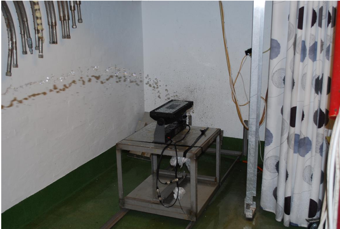
Photo 15. IPX5 During exposure.
