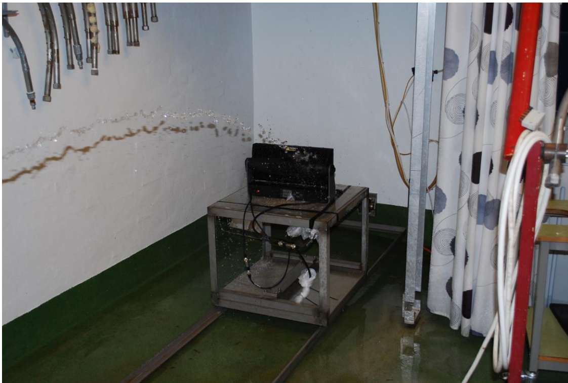
Photo 12. IPX5 During exposure.
