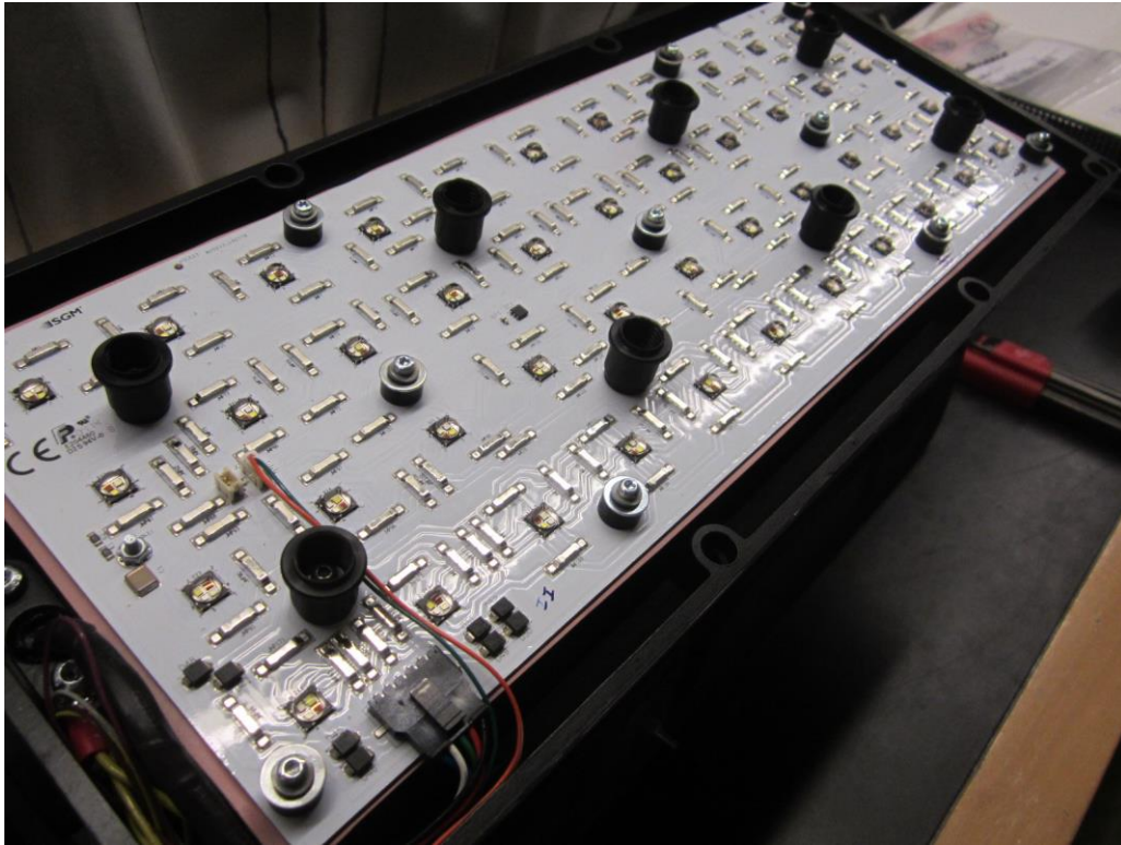
Photo 5. IP6X No dust observed inside the P-5 Wash Light.
