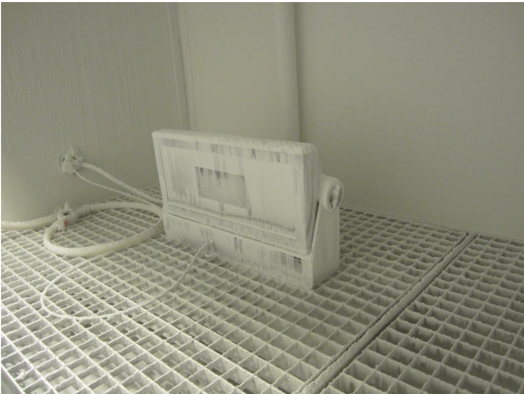
Photo 2. IP6X The P-5 Wash Light after exposure.
