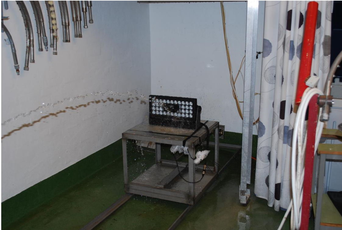
Photo 13. IPX5 During exposure.
