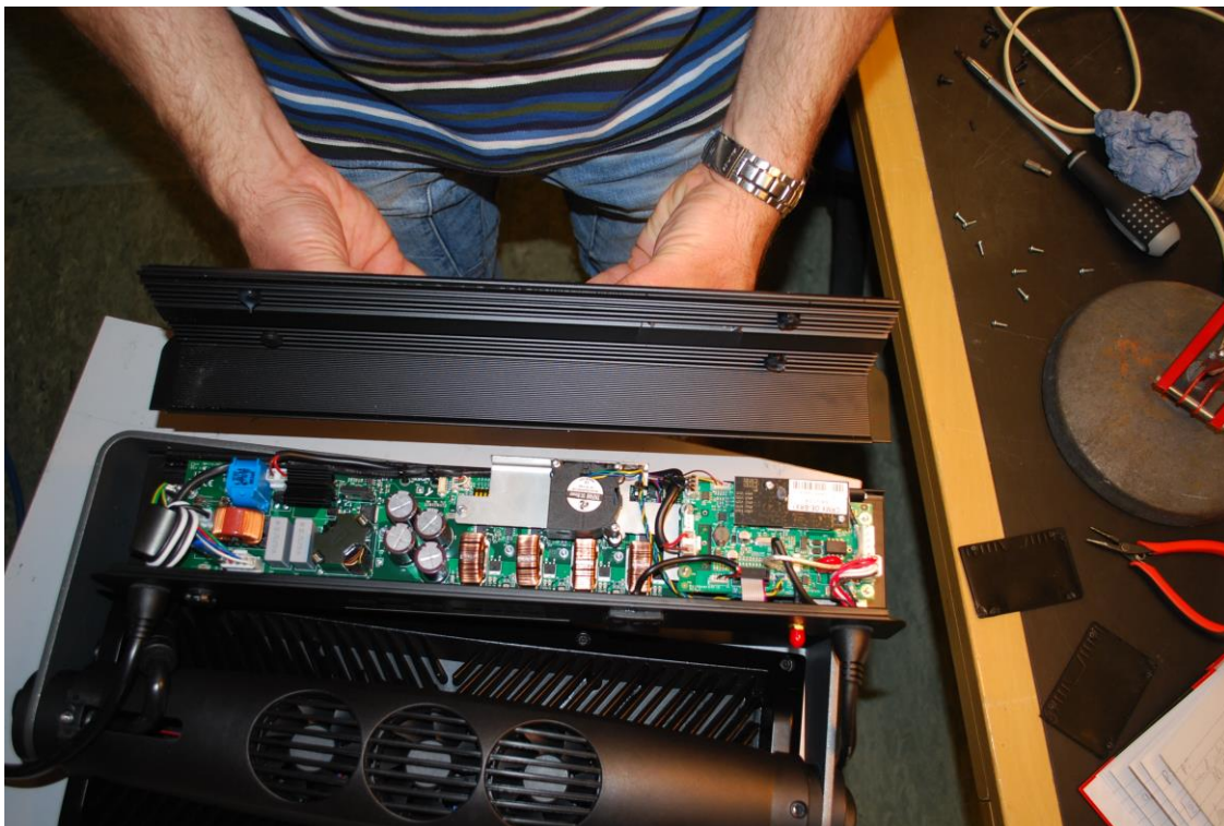
Photo 20. IPX5 No water observed inside the P-5 Wash Light.
