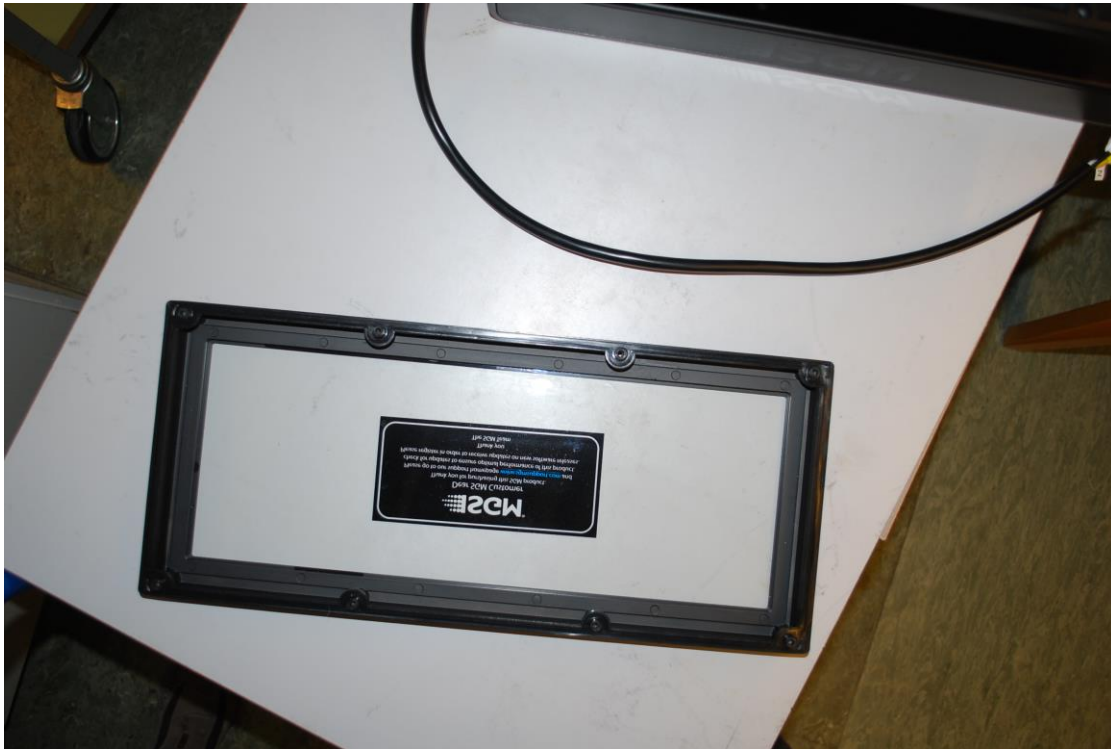
Photo 17. IPX5 No water observed inside the P-5 Wash Light.
