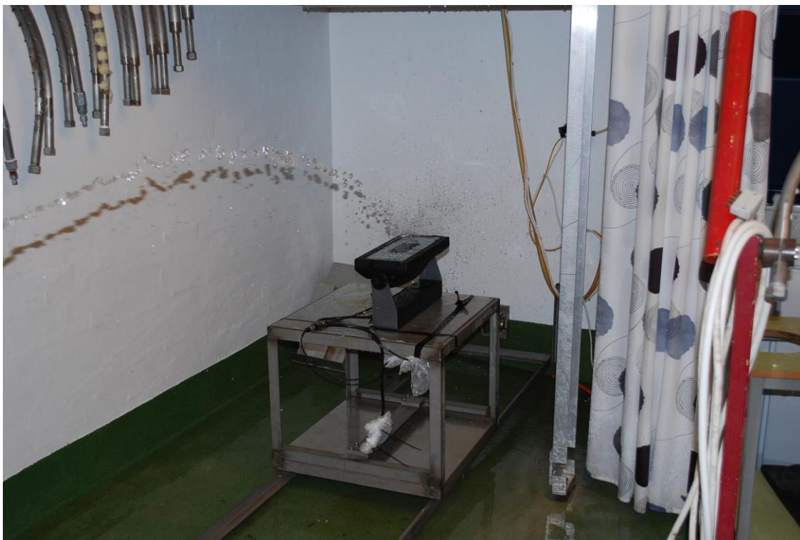
Photo 14. IPX5 During exposure.
