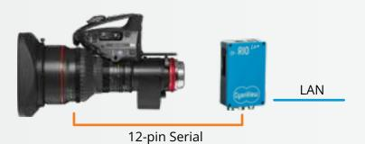
Canon CineServo have the same 12-pin connector as B4 lenses and control is done using the same cable and protocol.
