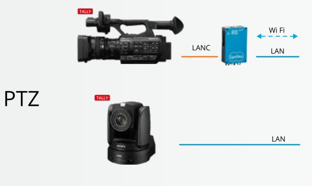
Handheld camcorders can be controlled over LANC. Newer models have built-in tally but an external box or LED can be added. The protocol is limited to exposure (iris, electronic ND, gain), menu navigagtion, record and tally. No color settings.
