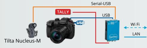
The Panasonic GH5S can be controlled over USB. External lens motors from Tilta or using C-Motion Broadcast Camin are supported. This is useful on gimbals or drones. An external tally box or LED can be connected to RIO directly.
