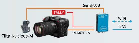
The C70 can also be controlled over Remote-A. An external tally light can be added on the camera hotshoe. Tilta motors or C-Motion Broadcast Camin can be used to motorize lenses.
