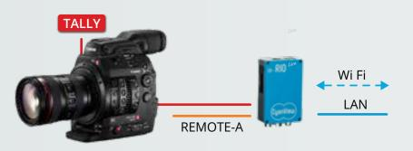
Control of the previous EOS-C models is done through the Remote-A 2.5mm jack port. This provides the same functionality as the RCV-100 remote. Most settings are controlled in relative mode which doesn't provide accurate readings of the camera settings.
