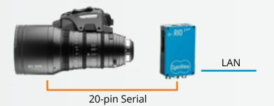
Fujinon lenses can be controlled directly through the 20-pin AUX connector using the CY-CBL-6P-FUJI cable and selecting the protocol named "B4 Fuji" in the interface. It is also possible to use the CY-CBL-6P-B4-01 combined with the Fujinon 20-pin to 12-pin cable and using the protocol named "B4 Generic" ivn the interface.
