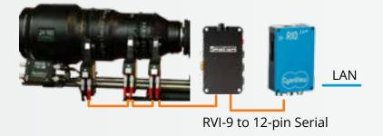
C-Motion supports the "B4 Generic" protocol. You need the C-Motion RVI-9 cable to allow serial control of the unit, and the CY-CBL-6P-B4-01 cable to link it to the RIO connector.
