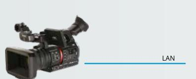
The CX Series provide the standard controls over IP: exposure, white and black balance. Menu navigation is possible so any other parameter can be configured that way. Tally isn't available though.
