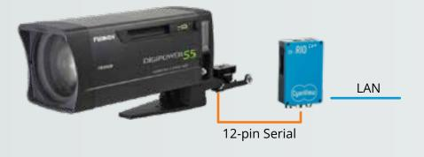
Box lenses can be controlled using the same "B4 Generic" protocol and CY-CBL-6P-B4-01 cable. Use lens support Fujinon ELH-112A-35A or Canon SUP-NS3 which both have a switch to select serial control instead of normal/parallel. The switch has to be in the serial position to get control. The old Fujinon ELH-112A-18A will require a wiring modification as they don't have the switch. Fujinon can provide the information though.
