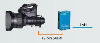
B4 lenses can be controlled using the CY-CBL-6P-B4-01 cable and selecting the "B4 Generic" protocol in the interface. Control is done use the serial protocol, not the analog lines so the lens has to support digital control.
