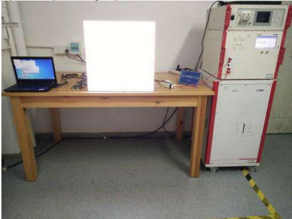
Photograph 9: Set-up for Voltage Dips on AC Mains
