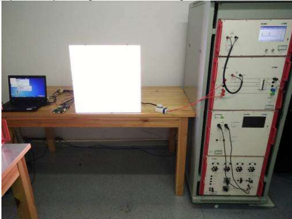
Photograph 8: Set-up for Surge on AC Power and Signal Ports
